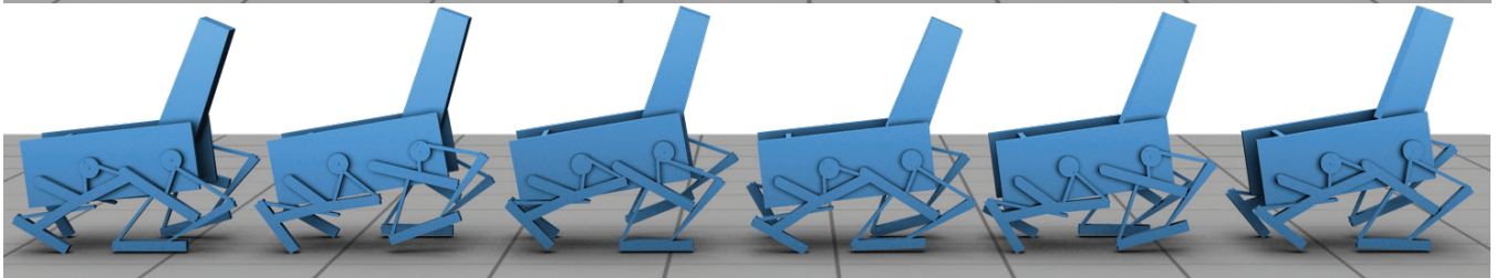
(c) Giraffe: Heavy neck makes the optimization adapt the automata-linkages accordingly.
