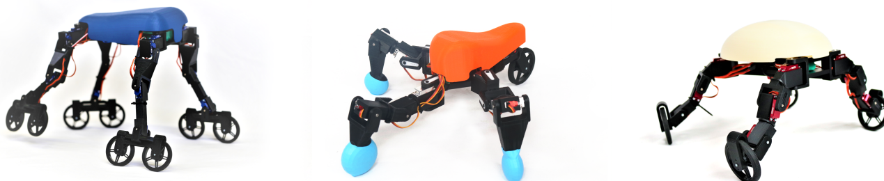
Fig. 1. Robotic creatures created with our computational design system employ arbitrary arrangements of legs and wheels to locomote.
