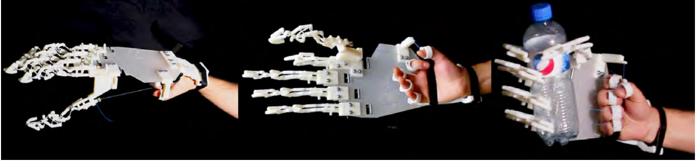
Fig. 12. Compliant Hand. A compliant finger mechanism is replicated and assembled to create a fully operational hand. Side and bottom views are shown on the left and in the middle. On the right we show the hand performing a teleoperated grasping task using cables for actuation. Thanks to restoring forces from the compliant flexures, the hand can be actuated using a single cable per finger.
