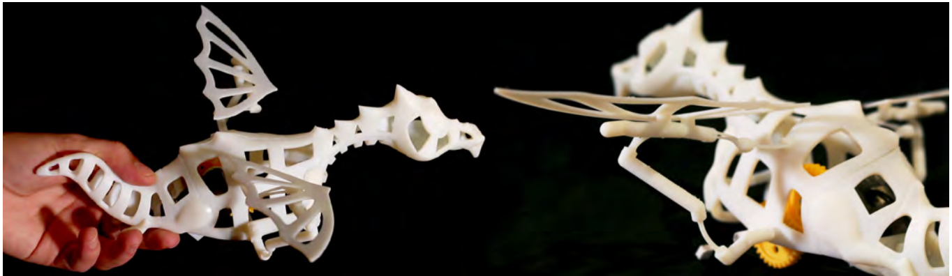
Fig. 13. Dragon . Full dragon (left) and close-up onto the wing mechanism (right). The wings of the dragon are two identical but mirrored versions of a spatial compliant mechanism. This example exhibits large deformations induced by twist, emphasizing the need for a twist-aware objective for preventing material failure.
