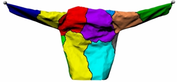
Fig. 4. Partitioning of a shirt for 12 processors.
