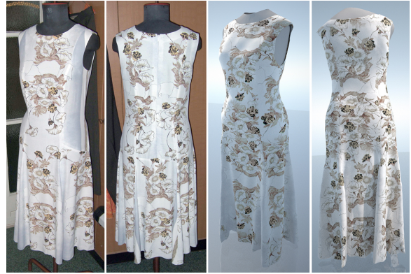
Figure 9: A comparison between a real garment and the simulation, using our proposed techniques and actual measured data for tensile and bending stiffness. The fabric bending coefficients are \{b_1 = 0.0973, b_2 = 0.0973, c_1 = 0.0453\} , and the fabric with interlining is simulated using \{b_1 = 0.5168, b_2 = 1.8856, c_1 = 2.2683\} .
