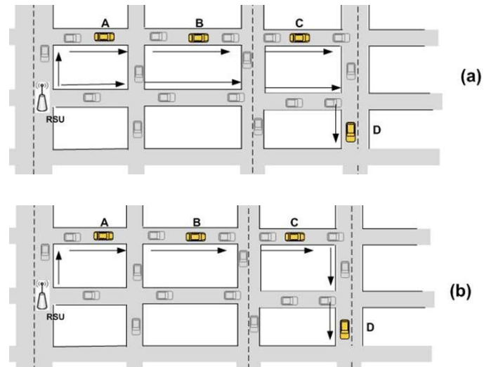
Fig. 6. Comparison between Shortest Path Tree and Min Steiner Tree: (a) Shortest Path Tree includes 8 busy street segments, (b) Min Steiner Tree includes only 6 busy street segments.
