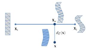
**Figure 2:** Artist-provided poses  $\mathbf{X}_1$  and  $\mathbf{X}_2$  specify a subset of desirable deformations. During simulation, a secondary potential energy term attracts the current deformed configuration  $\mathbf{x}$  to  $\mathbf{X}_w$ , its projection on the example-manifold. We represent the input poses, as well as  $\mathbf{X}_w$ , as a disconnected set of elements, which greatly simplifies our problem formulation.
