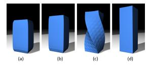
**Figure 4:** Different plasticity approaches illustrated on a vertically compressing cuboid (a) with a single twist example provided. Plastic deformation without examples (b), example-based plasticity with projection (c), and additional distance-dependent yield threshold (d).
