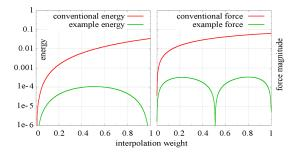
**Figure 3:** Left: energy landscape on the example manifold. Right: generalized forces due to weight variation.
