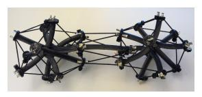
**Figure 8:** After two weeks, the 3D printed struts have deformed significantly under the tension of the cables.
