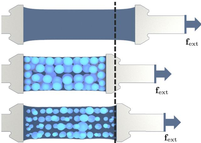
Fig. 4. Optimizing for desired displacement (*dashed line*) under a given force  $\mathbf{f}_{\text{ext}}$ . The homogeneous base material is too soft (*top*), whereas the initial inclusion distribution is too stiff (*middle*). After optimization, the target displacement is accurately matched (*bottom*).
