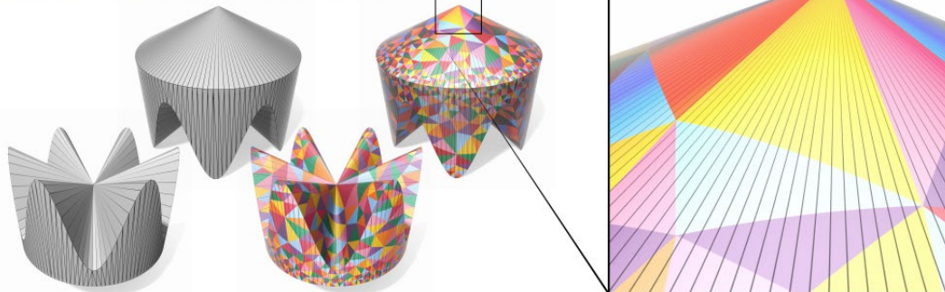
Fig. 1. Our data structure makes it possible to treat a crude input mesh (left) as a high-quality intrinsic triangulation (right) while exactly preserving the original geometry. Existing algorithms can be run directly on the new triangulation as though it is an ordinary triangle mesh. Here, a mesh with tiny input angles becomes a geometrically identical Delaunay triangulation with angles no smaller than 30^\circ —a feat impossible for traditional, extrinsic remeshing.
