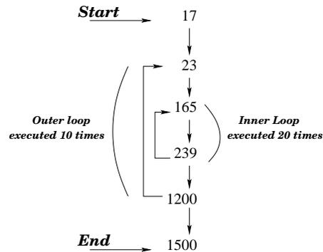
The memory addresses are in decimal. With the exception of the two branches at addresses 239 and 1200, all instructions utilize straight line sequencing. Each address contains one instruction. The program is to be run on a computer that has the following parameters :
