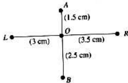
$$\left(\frac{\partial u}{\partial x}\right)_{L,0} = \frac{(u_0 - u_L)}{hL} \quad \left(\frac{\partial u}{\partial x}\right)_{0,R} = \frac{(u_R - u_0)}{hR}$$
