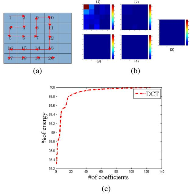
**Fig. 1.** Graphical representations of the spatiotemporal spectrum: (a) snake order; (b) the slicing spectral energy of DCT coefficients; (c) The percentage of average accumulated spectral energy of 3D DCT coefficients computed on about  $3 \times 10^5$  spatiotemporal volumes
