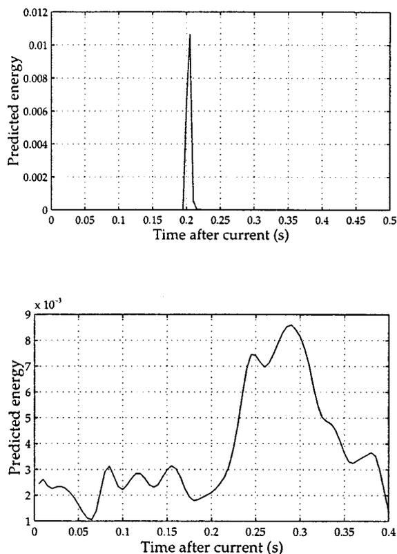
FIG. 7. Phase estimates, after tracking 5 s of a 2-Hz click track (top) and a polyphonic music example (bottom). The  $x$ -axis in each case covers the next full period of the resonator tracking the tempo, and the peak of the curve shows where the next beat is predicted to occur: about 210 ms in the future for the upper case, and 290 ms for the lower.
