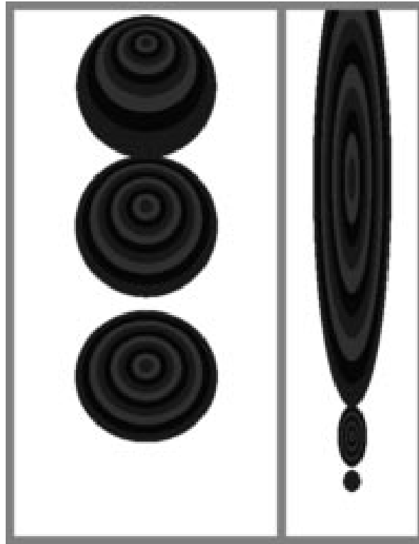
A Gaussian centered in texture space is not centered in screen space.
