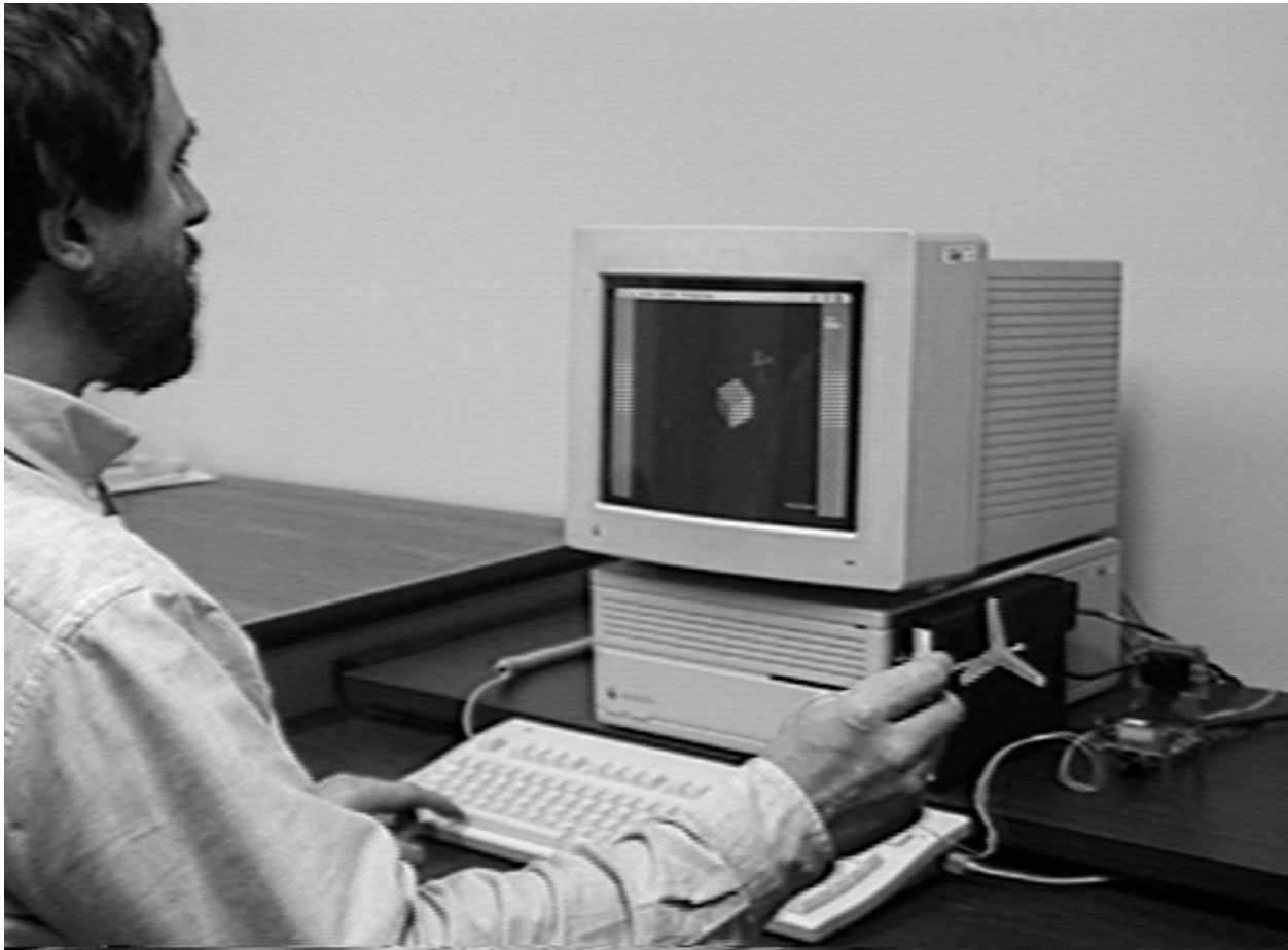
Figure 8: Video-based 3D mouse. The signal from the camera is sent to the black box at the right of the computer. This box detects the images of the light sources of the mouse and transmits their coordinates to the computer. The computer runs a driver based on POSIT.
