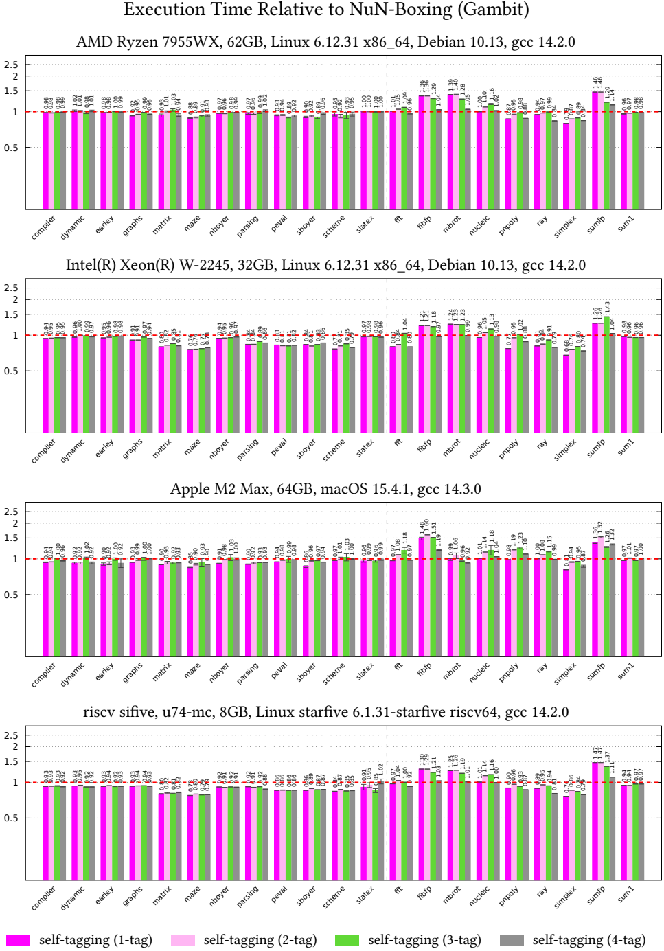
Fig. 8. Execution time of Gambit with each variant of self-tagging relative to NuN-boxing on four distinct microarchitectures (from top to bottom: AMD, INTEL, M2, and Risc-V). The y-axis shows execution time relative to NuN-boxing (dashed horizontal red line) on a logarithmic scale. 1.00x indicates no change, lower means faster, and higher means slower execution than NuN-boxing.
