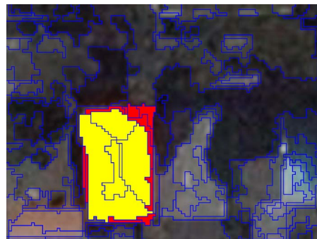
Fig. 1. Oversegmentation of roofs: Dark objects denote the background, yellow ones denote the foreground, and red ones are background objects that improve the rectangular segmentation of the foreground roof.
