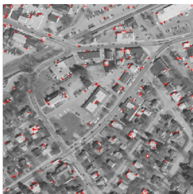
Fig. (d) Corner detection map based on multi-scale Harris operator for Fig.(b)
